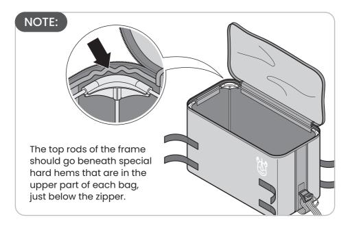
Secure the frame with four hook-and-loop flaps that go over the rods. Close the bag with the zipper.
