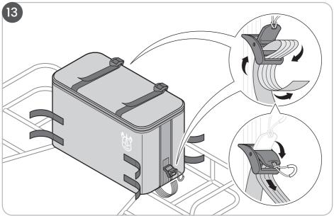
Connect the bags to one another using straps that have hook-andloop fasteners on them. When the bags are connected, the lids of the side ones should be opening outwards (away from the middle bag), and the reflective logos should be facing outwards, too.
